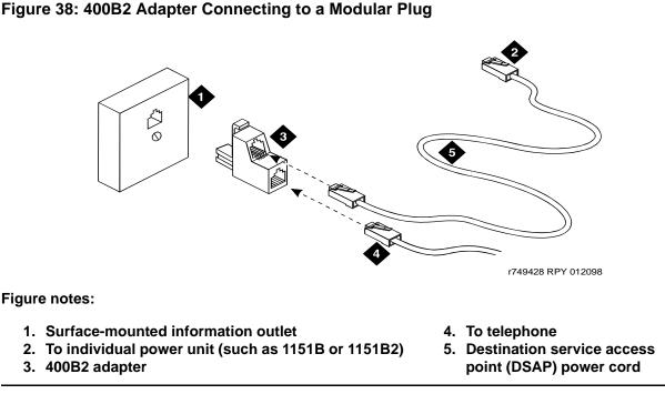
Adjunct power can be provided from the equipment room or equipment closet with 1145B power unit. The AUX connector (J1) on the processor interface cable can provide power for 1 attendant console. See <u>Table 36</u>: <u>Processor Interface Cable Pinout</u> on page 165.
